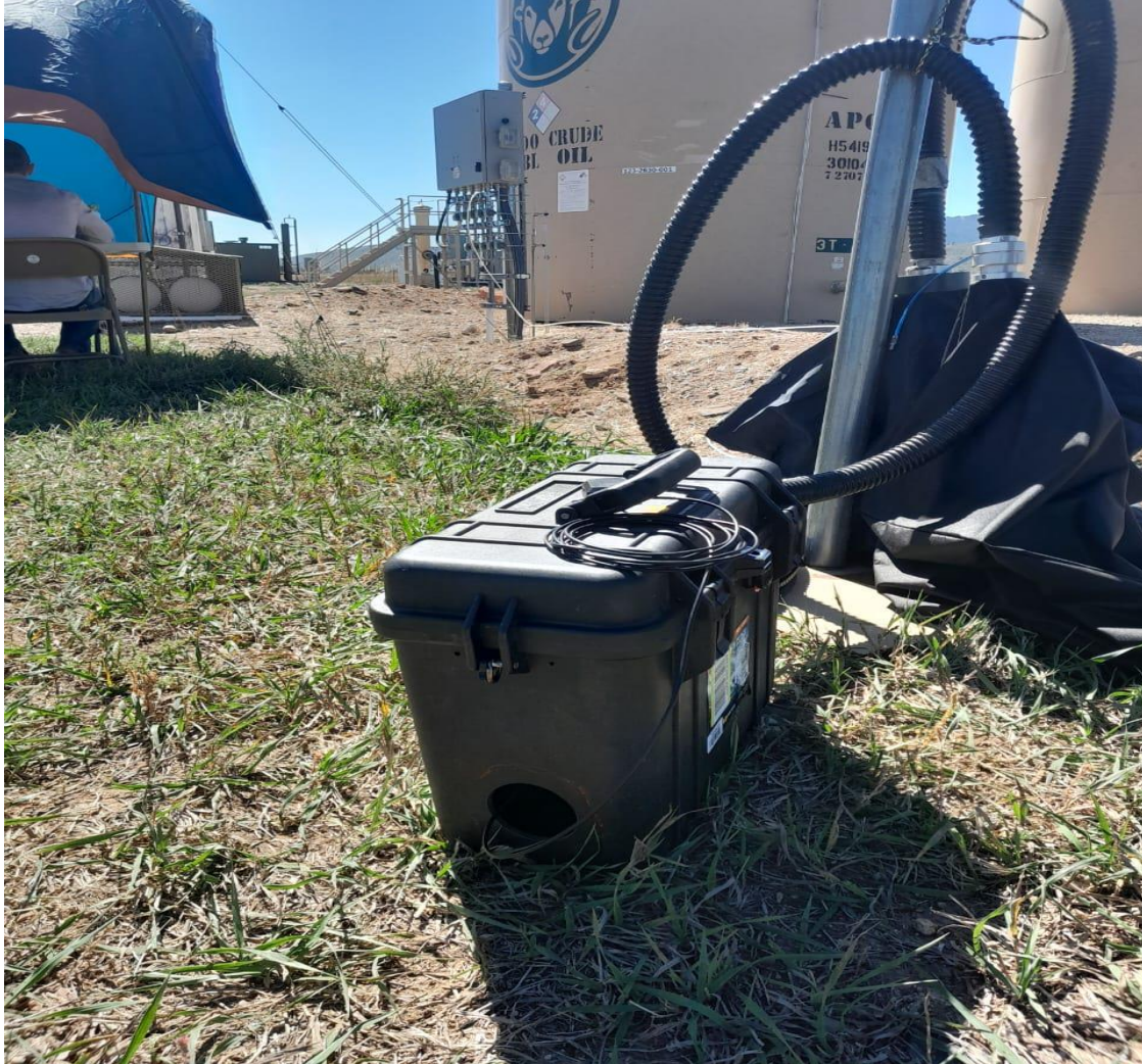
Figure 2: Accuracy Over Range test at METEC Facility with Colorado State University Open Source High Flow Sampler
