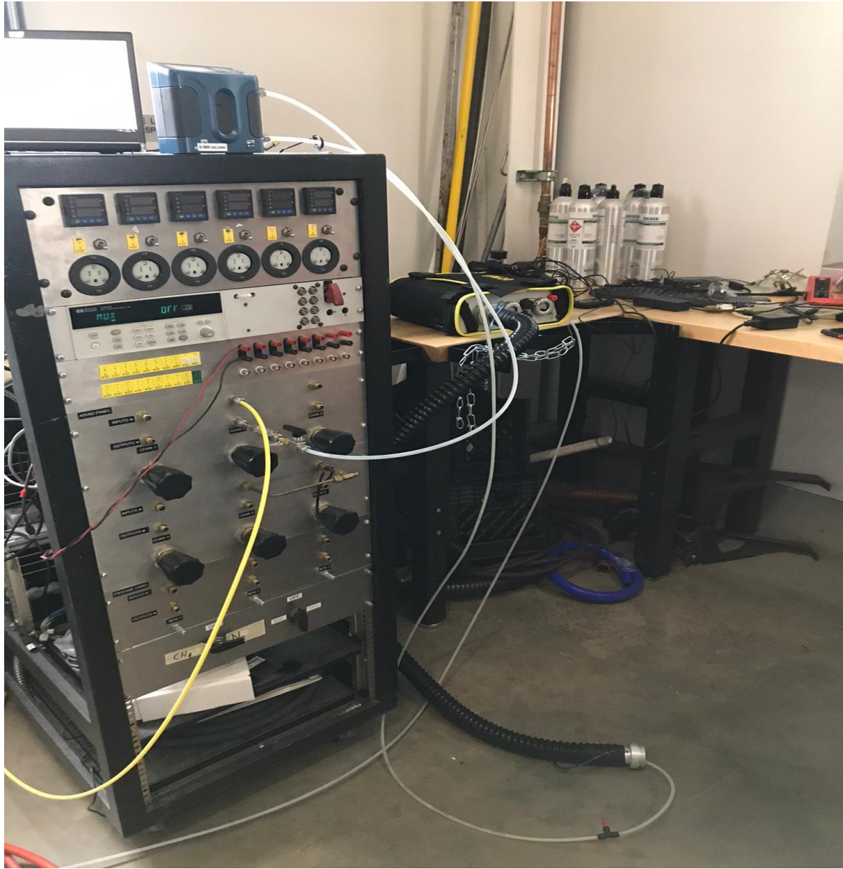
Figure 1: Air Flow testing of Gas Flow Meter 2.0 at the Powerhouse Energy Campus.
