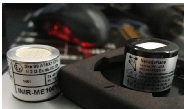
Figure 16: The SGX INIR-ME100 and Nevada Nano MPS Flammable Gas Sensor were chosen for use in the prototype OS-HFS.
