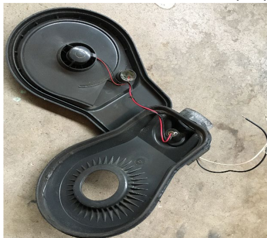
Figure 12: Inside the 3M GVP-100 blower motor used in the BHFS. The blower is certified for use in hazardous areas. All the internal electrical connections are encapsulated. The internal housing (upper left) is characteristic of a centrifugal blower design.
