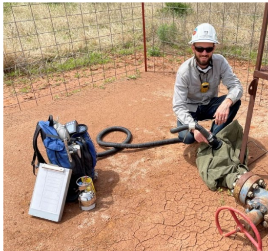
Figure 5: A BHFS is used to measure an emission on a wellhead.
