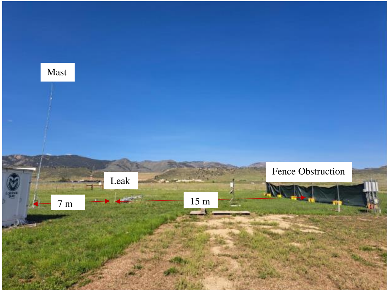
Figure 1 Aboveground set up for Experiment 1 CH 4 measurements conducted at METEC's rural testbed. The CH 4 sampling mast was located 7 m from the leak center, the mast has sampling heights at 0.5, 2, 5, and 7 m. The fence obstruction was located 15 m from the leak center. The obstruction height was set at 1.7, 1.5, 1.1, and 0.8 m to understand the effect of the obstruction on aboveground plume detection.
