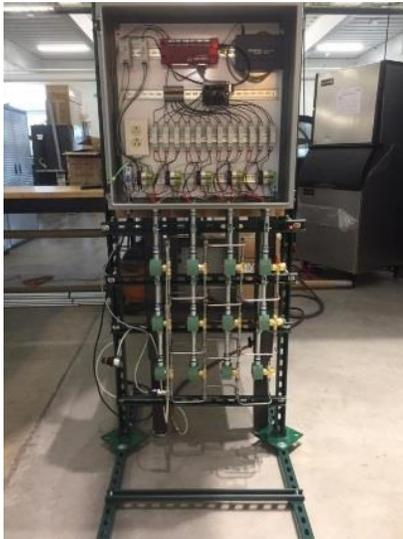
subsystems are each capable of controlling multiple source locations, independently or simultaneously, to produce steady or intermittent emission sources ranging from 2 SCFH to 300 SCFH. The control units will monitor gas pressures, temperatures and flowrates, and regulate gas releases remotely using
